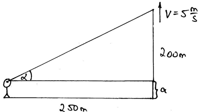
$$\alpha(t) = \arctan \frac{5 \frac{\text{m}}{\text{s}} \cdot t - a}{250 \text{m}}$$
